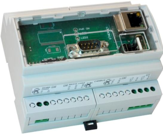
DANCE is an electronic device aimed for the monitoring of the status, measures and operations of a genset, tower light a tank, ecc... via **ETHERNET TCP/IP**.
